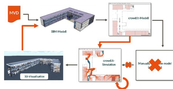
Figure 4 Schematic overview of the automated integration of people flow simulations into the planning process, after completion of the BEYOND project.
