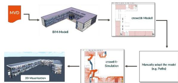
Figure 3 Schematic overview of the automated integration of people flow simulations into the planning process, after completion of the AHEAD project.
