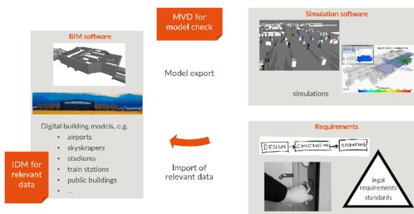
Figure 2 Overview of the future integration of fire protection into the BIM planning process
