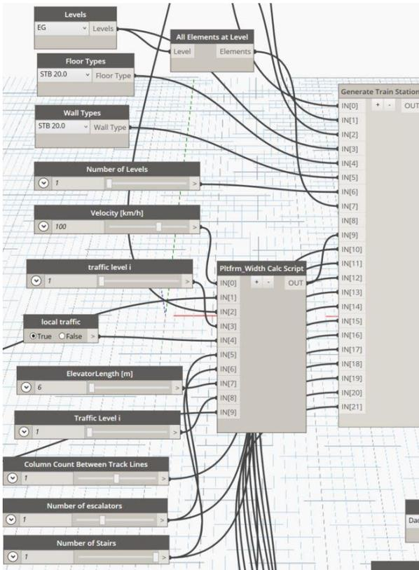
Figure 5 Example parameterization in Dynamo
