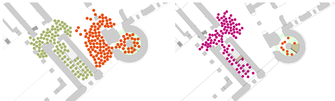
Figure 6: Left: Congestions, occurred in front of the staircases during the first iteration. Right: Congestion in front of staircase during the second iteration.
