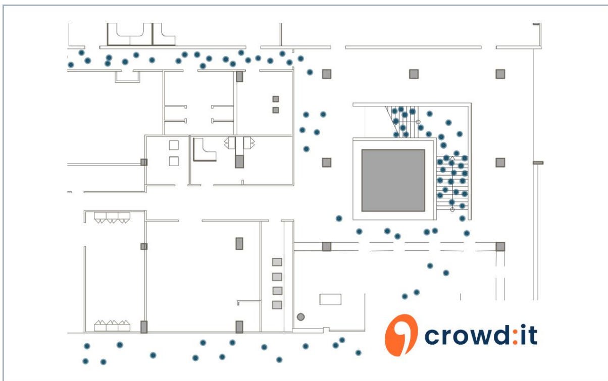
Figure 1: Snippet from the simulation software crowd:it , including a floor plan and blue circles representing the position of individual agents.
